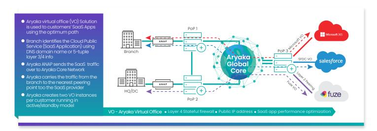
The solution leverages the power of Aryaka PoPs, by configuring them as virtual offices VOs. Two VO instances are created per customer running in active / standby mode. These VOs act as an exit point from Aryaka PoP to the Cloud Application, breaking out the traffic from the secure Aryaka backbone.
