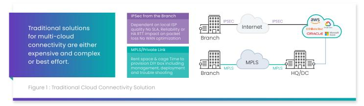
Traditional cloud connectivity solutions rely on either IPSec through the Internet or private MPLS links, neither of which address the multi-cloud challenge for fast, reliable and easy to manage connectivity.
