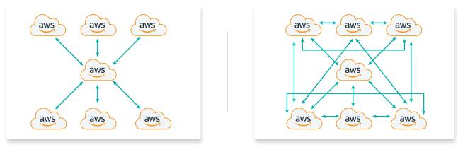
Traditional solutions for this connectivity has relied on partially meshed or fully meshed (VPC Peering). The drawback with these solutions is that these peering connections often require modifications to the associated VPCs' route tables and, as the number of VPCs grows, this can be difficult to maintain. Furthermore, there is a limitation of a maximum of 125 peering connections per VPC.
