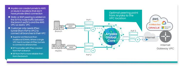
Aryaka's network connects all the branches using a single IPSec tunnel going from the PoP to the cloud provider's VPC. This architecture is far superior to the traditional SD-WAN architecture, where a single VPC has a number of IPSec tunnels to connect the branches. Advantages of this solution include better reliability and a smaller Round trip time (RTT).
