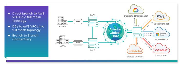
Aryaka with its PoP architecture simplifies multi-cloud connectivity. The PoP closest to the laaS location acts as the transit point for the inter-cloud traffic by providing an efficient alternative to traditional solutions.
