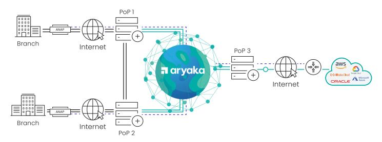
In the spirit of flexibility and agility that is so synonymous with cloud offerings, Aryaka provides two different ways to connect to IaaS providers. The first is a direct connection that adheres to AWS's Direct Connect, Google's Dedicated Interconnect and Alibaba Cloud's Express Connect, Microsoft's ExpressRoute or Oracle's FastConnect, and the second is an IPSec tunnel from the nearest PoP router.
